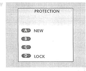
Enter the current password (new or default) on the dialing keypad to access protection parameters.
